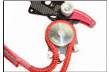
3. Press the rope into the recess in the drum and then lay the rope in-between the two bottom guides.
