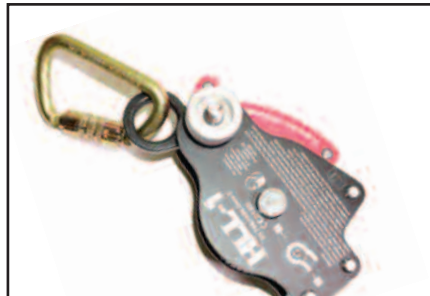
5. With a min 30kN carabiner and strop as required attach the eye of the rope to one anchorage, with a second carabiner on the cam of the tensioner secure this to the second anchorage.
