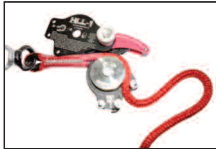
2. Wrap the anchor end of the rope around the drum, taking note of the diagram.
