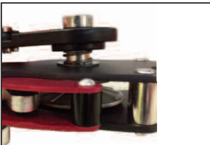
7. Compress the tension handle towards the device, whilst turning to align the square drive, and hold in place.
