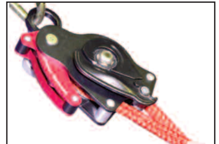
6. Pull initial slack through the tensioner by hand, check that the rope is sitting in the groove of the drum at this time. If the rope is trapped between the cam and the side of the drum, release the cam by hand and pull on the rope till it slips back into the centre of the drum.
