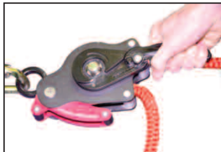
8. To achieve correct system tension, unfold the tensioning handle, compress the centre of the arm and turn in an anti-clockwise direction until the lifeline becomes taught enough to hold and arrest a fall or the rope begins to slip. Do not force the handle. Do not try to reverse wind the tensioner, the cam will lock and resist any rotation in this direction. Check that the hand nut is tight.
