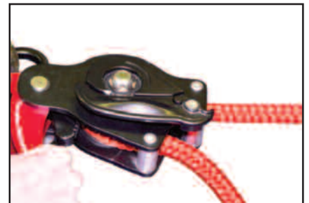
9. Decommissioning is easily achieved by partially loosening the hand nut and pulling back the tension release lever, allowing the rope to slip through the device. Warning: Ensure the handle is disengaged allowing the shaft to rotate independently from the handle arm before releasing tension. On releasing the rope check the rope at the point of the tensioner to ensure that wear and tear during use has not separated the fibers of the rope's protective sheath.
