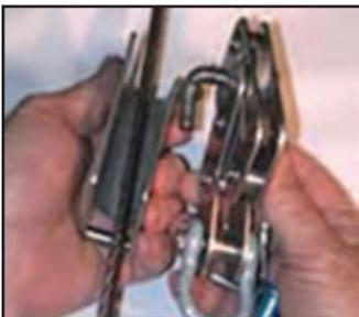
3. Place rope grab on rope with direction arrow pointing up.
