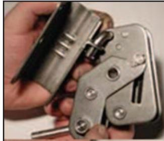
2. Swing cam and level-assembly up and open.
