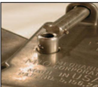
5. Make sure that locking pin balls appear on outside of main assembly.
