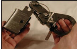
2. Swing cam and level-assembly up and open.
